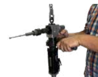
Pistol grip at back side with handle on left
