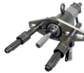
REAMMING Safely ream tube sheets.
