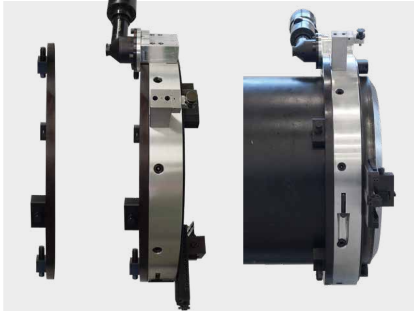
SFSF-1624 with ORR mounted on the 24" pipe schedule 120.
